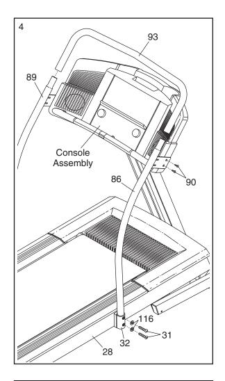
5. Attach the Upper Handrail (93) to the Left and Right Handrails (86, 89) with four 3/4" Tek Screws (91) (only two are shown); start all four Tek Screws before tightening them.
